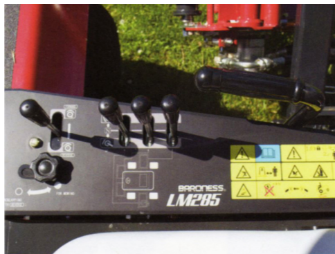
Right Dynamic brake, lock valve, outer units lock latch.
