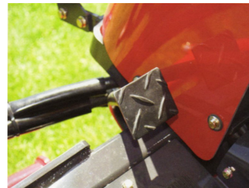
Right Dynamic brake, lock valve, outer units lock latch.
